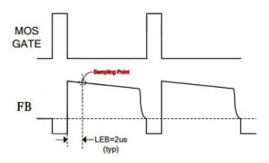
Figure 5. Feedback voltage detection
