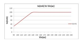
Figure 4. Io - Vin relation curve
